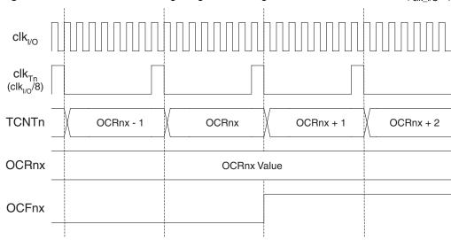
Figure 50. Timer/Counter Timing Diagram, Setting of OCF1x, with Prescaler (fclk 1/O/8)
