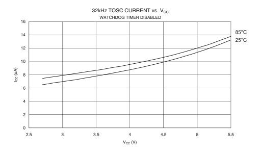
Figure 210. Watchdog Timer Current vs.  $V_{\text{CC}}$
