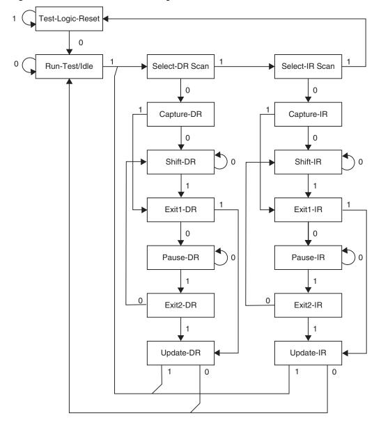
Figure 113. TAP Controller State Diagram
