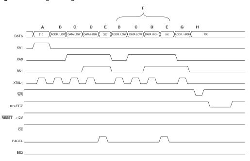
**Figure 129.** Programming the Flash Waveforms<sup>(1)</sup>
