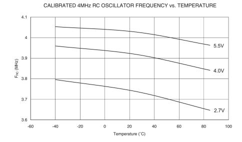
Figure 198. Calibrated 4 MHz RC Oscillator Frequency vs.  $V_{\rm CC}$
