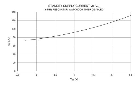
Figure 173. Standby Supply Current vs. V<sub>CC</sub> (6 MHz Xtal, Watchdog Timer Disabled)
