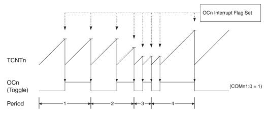
An interrupt can be generated each time the counter value reaches the TOP value by using the OCF0 Flag. If the interrupt is enabled, the interrupt handler routine can be used for updating the TOP value. However, changing TOP to a value close to BOTTOM
