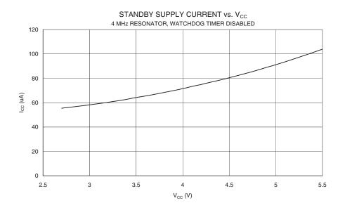
Figure 171. Standby Supply Current vs. V<sub>CC</sub> (4 MHz Xtal, Watchdog Timer Disabled)
