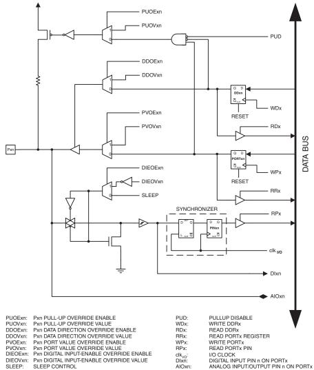
1. WPx, WDx, RRx, RPx, and RDx are common to all pins within the same port. clk<sub>I/O</sub>, Note: SLEEP, and PUD are common to all ports. All other signals are unique for each pin.
