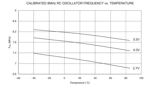
Figure 195. Calibrated 8 MHz RC Oscillator Frequency vs.  $\rm V_{\rm CC}$
