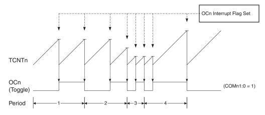
An interrupt can be generated each time the counter value reaches the TOP value by using the OCF2 Flag. If the interrupt is enabled, the interrupt handler routine can be used for updating the TOP value. However, changing the TOP to a value close to BOTTOM when the counter is running with none or a low prescaler value must be done with
