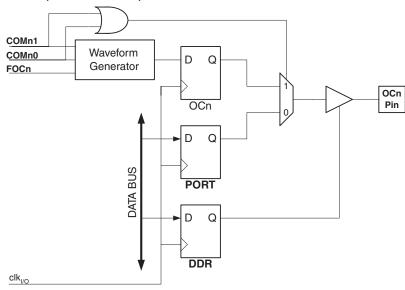
Figure 30. Compare Match Output Unit, Schematic
