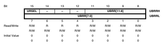
The UBRRH Register shares the same I/O location as the UCSRC Register. See the "Accessing UBRRH/ UCSRC Registers" on page 163 section which describes how to access this register.
