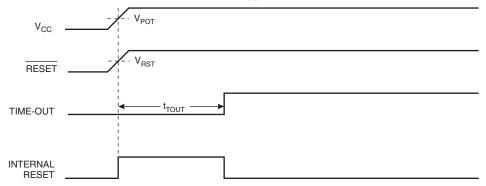
Figure 17. MCU Start-up, RESET Extended Externally
