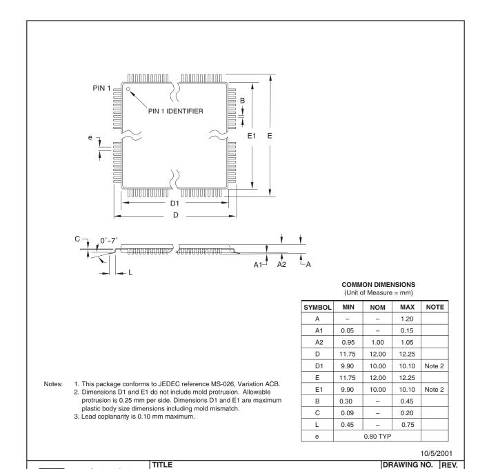
44A, 44-lead, 10 x 10 mm Body Size, 1.0 mm Body Thickness,
