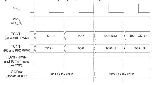
Figure 51. Timer/Counter Timing Diagram, no Prescaling
