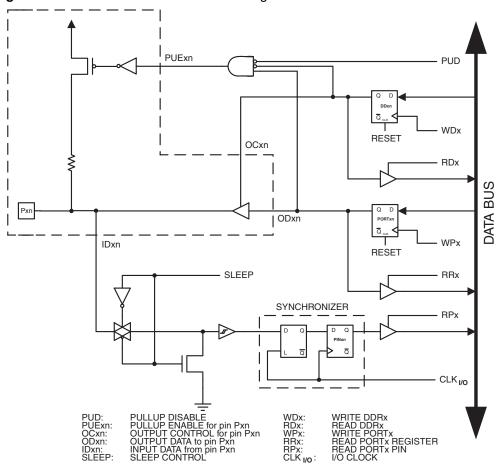
Figure 117. General Port Pin Schematic Diagram<sup>(1)</sup>
