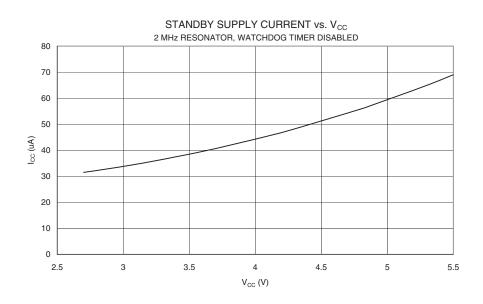
Figure 169. Standby Supply Current vs. V<sub>CC</sub> (2 MHz Xtal, Watchdog Timer Disabled)
