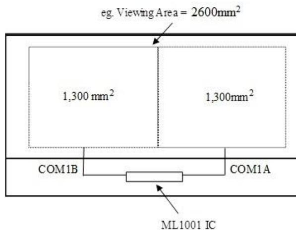
*Note : COM1A and COM1B shall cover half of the Viewing Area (ie. Area = 1,300mm<sup>2</sup>)
